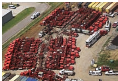
Figure 1 Shale gas frac job with hydraulic truck array, Barnett Shale, Texas. Courtesy: http://www.barnettshalenews.com .
